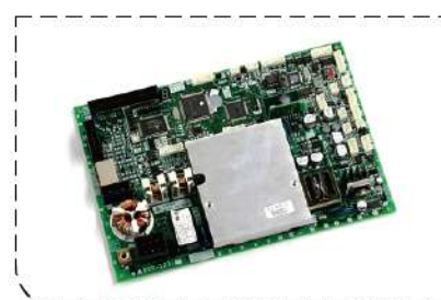
DOR-1231 Mitsubishi door machine board
